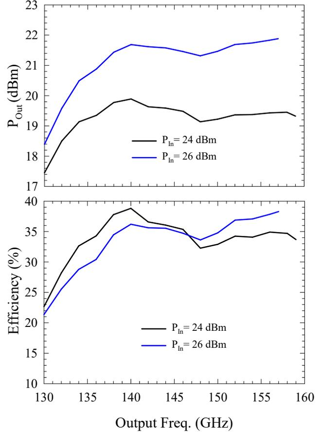
Fig. 3. Experimental output power (a) and efficiency (b) of the doubler from 130 to 160 GHz. The results are obtained with 24 dBm (black line) and 26 dBm (blue line) fixed input power.
