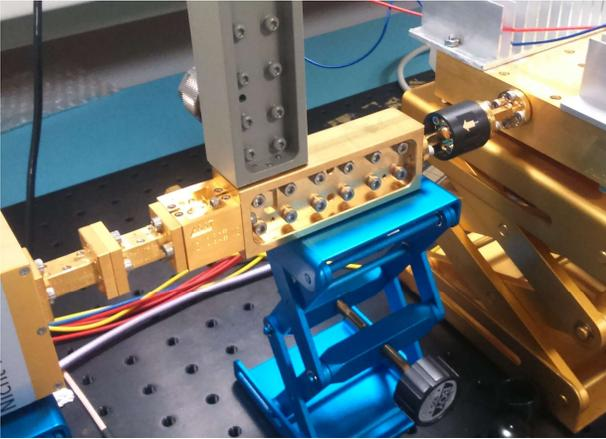
Fig. 2. Experimental setup to characterize the 135-160 GHz doubler developed at ACST.
