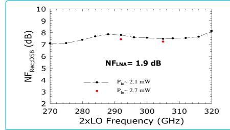
\*The NF is given including the noise figure of the LNA used for test.
